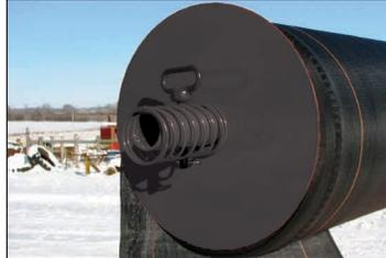
**FABRIC TENSION SPRING AND 16" DIAMETER FABRIC PLATES**
